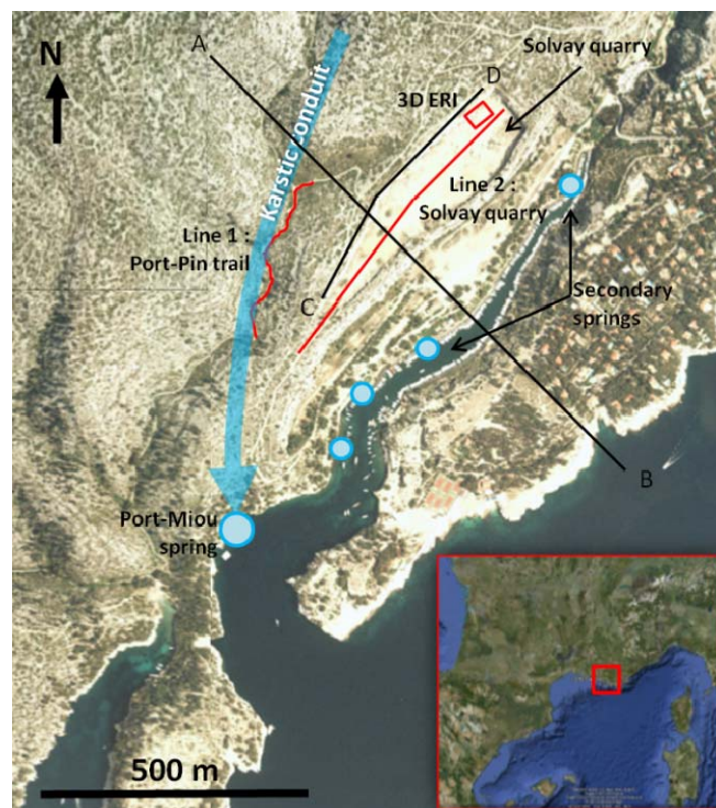
Figure 4- 35 : Figure 1 : Location of the study area. In red, the 2D and 3D ERT surveys. The blue arrow localizes the explored karstic conduit. The blue circles point coastal springs. Geological sections AB and CD are reported on the map.
